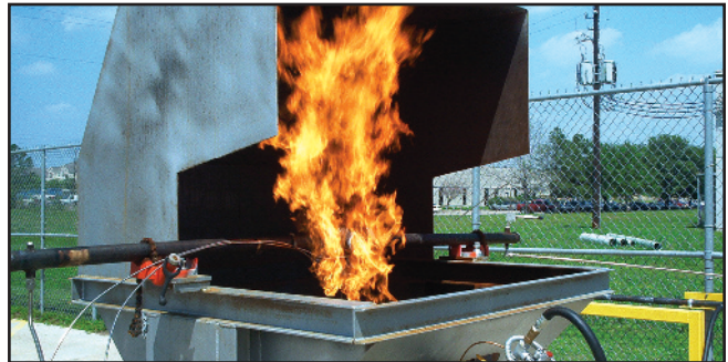
All Series 5312 valves meet API 607 firesafe standards.
