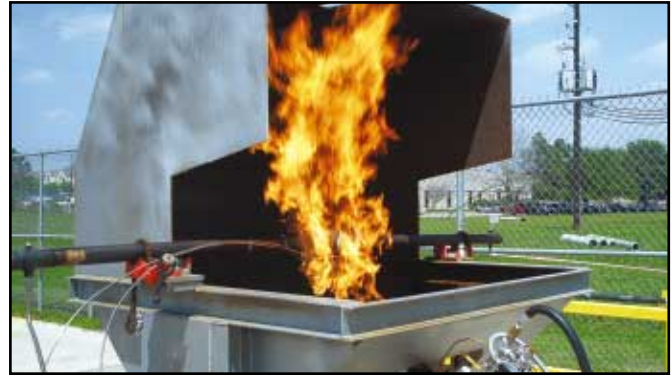
All Series 5312 and 5322 valves meet API 607 Firesafe standards.
